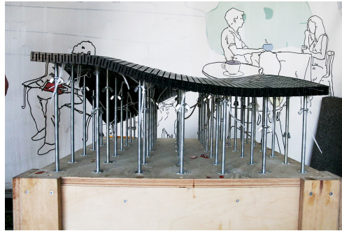
Figure 1 FlexiMold Flexible Formwork Device.
