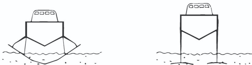
Figure 1.1: A hydrofoil vessel with surface piercing foils on the left and a hydrofoil vessel with fully submerged hydrofoils on the right. Figure based on [25].
