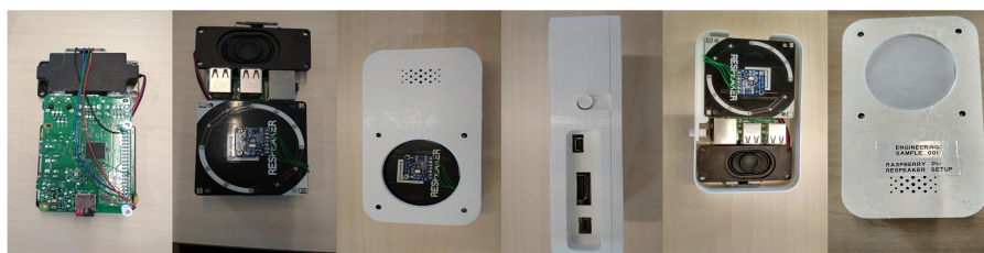
Figure 4.2: The respeaker and Raspberry Pi setup. The setup was enclosed in a 3D designed box to prevent contact with the components and mishandling and damage of the components.
