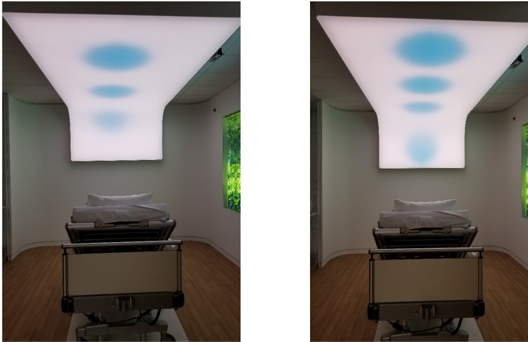
Figure 3.6: Testing the position of the circle at different places in the VitalSky. In the left figure it can be seen that the content on the curve is much more blurred than the rest. The circle was placed below the curve on the figure on the right. The circle below the curve is still blurred but less than the circle at the curve.
