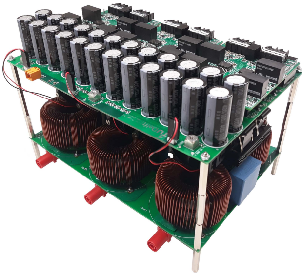
Fig. 15. Prototype of the 10-kW 2L-VSC used for the efficiency testing of the mcHyS with an LCL filter in the bottom.
