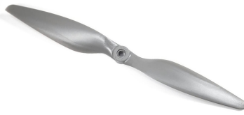
(b) 18*8 propeller produced by APC. a
