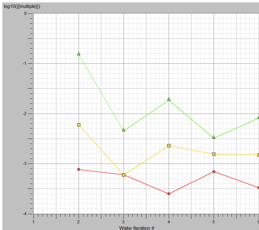
Figure 12.5: Convergence of \frac{L}{D} , C_L and the C_D in the OpenVSP VLM analysis.
