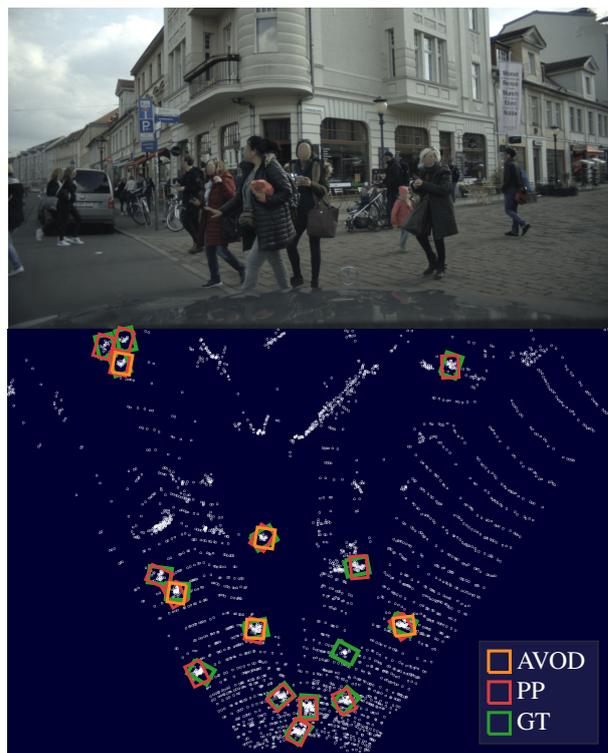
Fig. 1. An example of the predicted bounding boxes of PointPillars [6] (PP) and AVOD [7] on a scene from the EuroCity Persons 2.5D [8], along with the annotated ground truth (GT).
