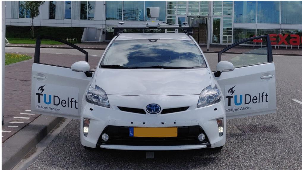
Figure 1.1: The TU Delft Toyota Prius. This car is equipped with different types of sensors, one can observe a LiDAR on top of the car. The car is also equipped with stereo cameras and radars. (Adapted from Palffy [41])
