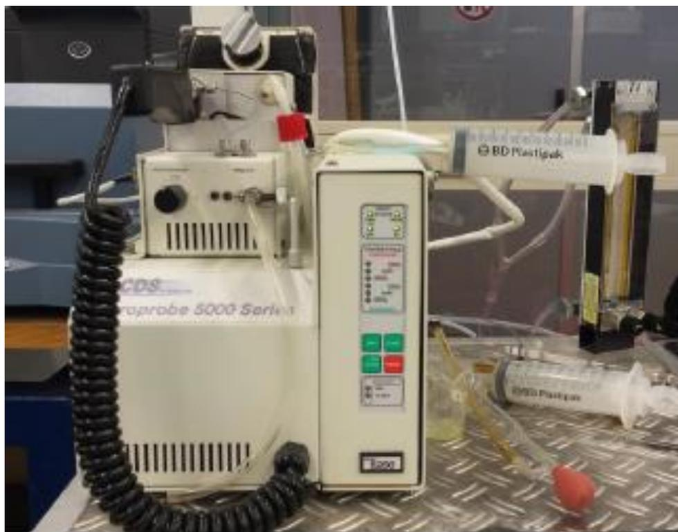
**Figure 2.1:** CDS Pyroprobe 5200 setup during a fast pyrolysis experiment
