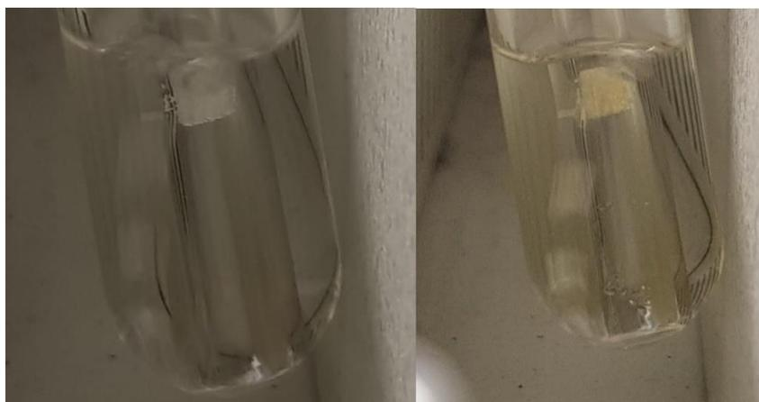
**Figure A.2:** On the left the isopropanol filled condenser before the initiation of a Miscanthus fast pyrolysis experiment at 900 °C. On the right the condenser after the completion of the same experiment
