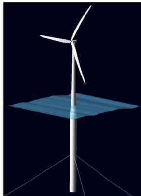
Figure 3.4: A visualisation of the OC3-Hywind concept with a 5MW wind turbine, retrieved from [45].
