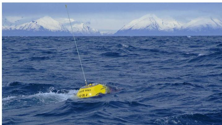
Figure 2.6: A Datawell directional waverider buoy deployed by the Hydrographic Institute of the Republic of Croatia. Retrieved from [52].
