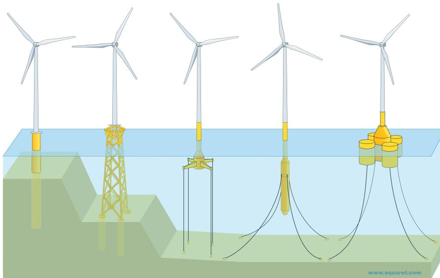
Figure 1.2: Types of foundations and moorings for bottom fixed and floating offshore wind turbines. From left to right: Monopile, Jacket, TLP, Spar, Semi-submersible [5].
