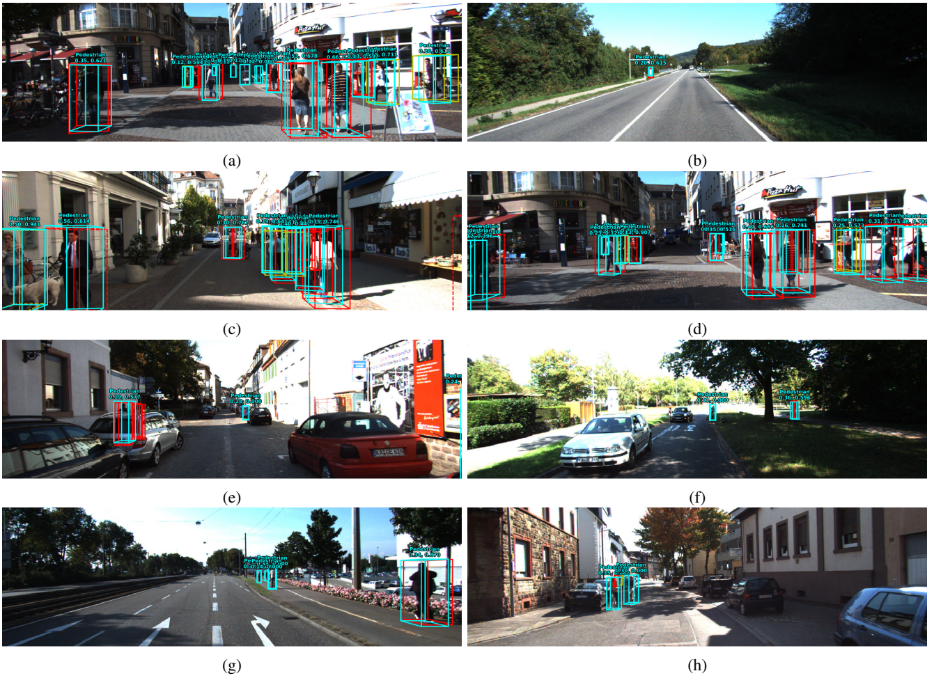
Fig. 3: Qualitative results for the proposed model on the KITTI validation set. The model can estimate the 3D location of people with different orientations and poses. (a) - (d): examples with good performance on crowded scenes, far away objects, occluded and truncated objects. (e) - (h): failure cases with missed detections, false positives and confusions with cyclists. Ground truth: red. Predictions: cyan. Numbers on top of boxes: detector objectness, IoU.
