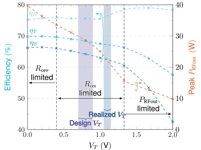
Fig. 8. Theoretical full power-DTX performances for the optimized class-BE designs for varying values of  $V_T$  of the applied LDMOS technology. The design parameters used to generate this graph are:  $L_{\text{bond}} = 0.6$  nH,  $R_{\text{bond}} = 0.2$   $\Omega$ ,  $Q_{L_0} = 10$ ,  $k_m = 0.2264$ ,  $f_0 = 3$  GHz,  $d = 50\%$ , and  $V_{\text{Ch}} = 2.5$  V; the remaining parameters depend on  $V_T$  and are given in Table I.
