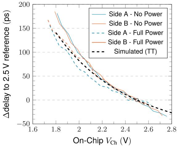
Fig. 17. Change in propagation delay of the CMOS tapered buffer chain compared to the  $V_{Ch} = 2.5$  V reference case versus the measured  $V_{Ch}$ , which includes the  $IR$ -drop (averaged measurements, and the  $\pm 1\sigma$  measurement variation is 14.4 ps). Thick dashed line: the simulated propagation delay.
