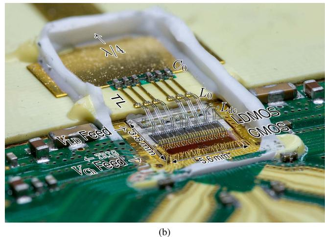
Fig. 9. Realized power-DTX configured for polar operation with the single-ended 2.1-GHz class-BE output matching. The prototype features a CMOS 40-nm controller and a  $V_T$ -shifted segmented LDMOS output stage, featuring two switch banks that take their ACW data from time-multiplexed on-chip memory. The power-DTX prototype also has extra trigger output pins to monitor its output independent of the LDMOS die. (a) Schematic. (b) Photograph with the ceramic cap removed.
