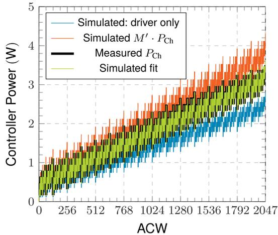
Fig. 10. Simulated drive power including  $C_{dr,o1}$ , this power is multiplied by the theoretically calculated  $M' = 1.532$  to provide the total power consumption of the driving drive chain, which is compared to its actual measured values.
