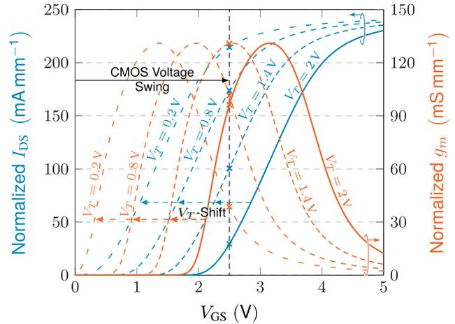
Fig. 2. LDMOS  $I_{DS}$  and  $g_m$  curves normalized per mm when  $V_{DS} = 28$  V for different  $V_T$ -shifts to lower voltage levels (shown in dashed line). The solid lines illustrate the nominal LDMOS technology as typically used for analog base station implementations.
