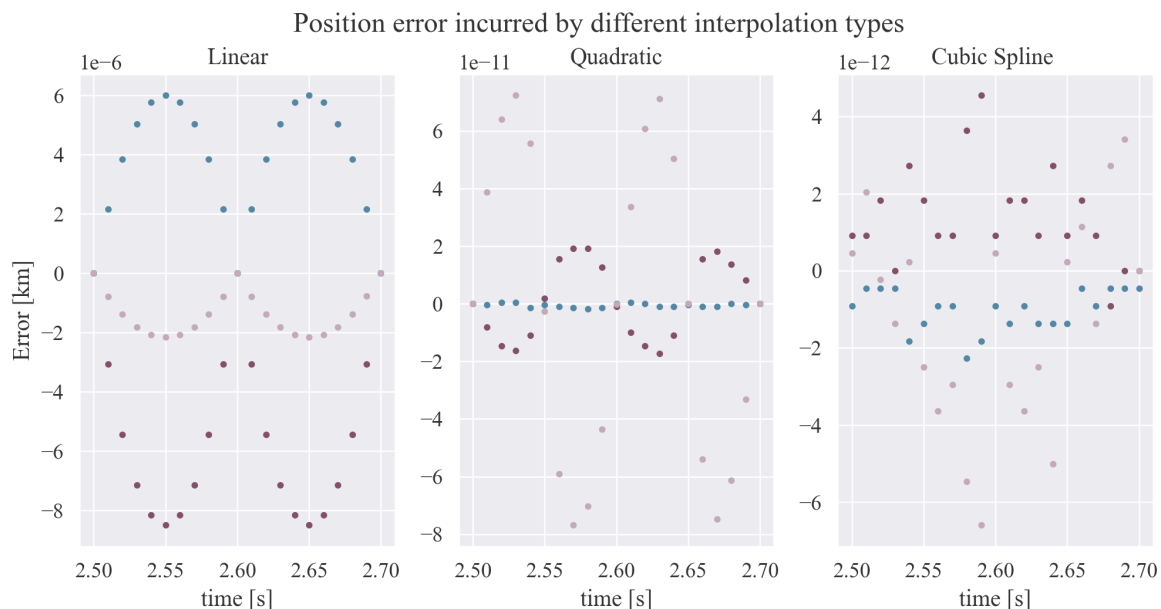
Figure 7.6: Error incurred by linear, quadratic and cubic spline interpolation for a set of data points between the interpolated position of the catcher of the satellite and the position obtained through the Kepler solver for the x, y, z components.
