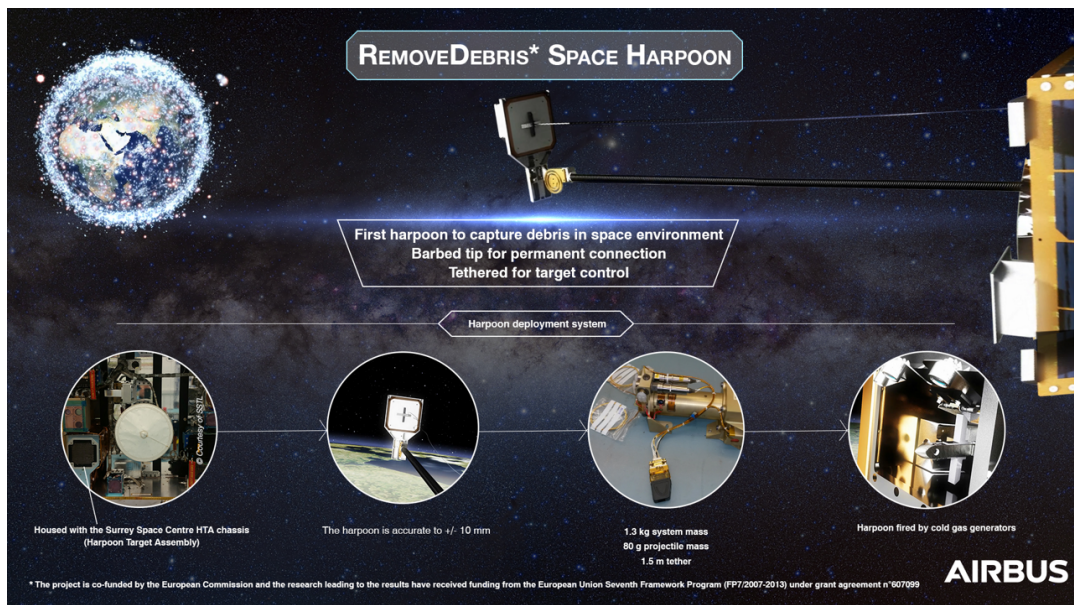
Figure 4.9: Illustration of RemoveDEBRIS ADS Harpoon concept (Airbus, 2021).
