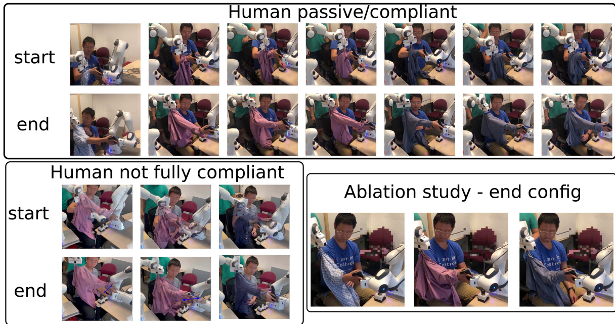
Fig. 15. Starting and/or end configurations for three different experiments: 1) human passive/compliant, 2) human not fully compliant, and 3) the ablation study where the human remains static. For experiments where the human is not fully compliant, we also display with high transparency a nominal end configuration when the human is compliant. The deviation from the nominal end configuration is indicated by a blue arrow.
