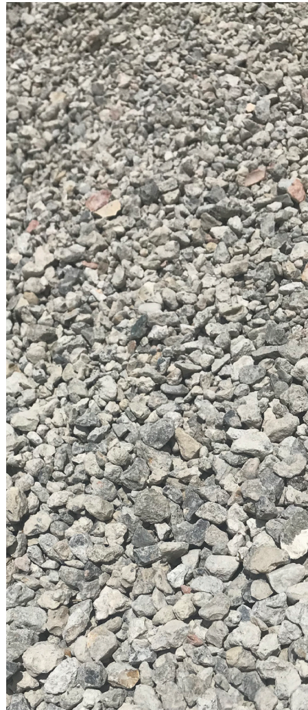
Gravel Concrete waste from demolished parts of the Molenpoort Shopping Mall
