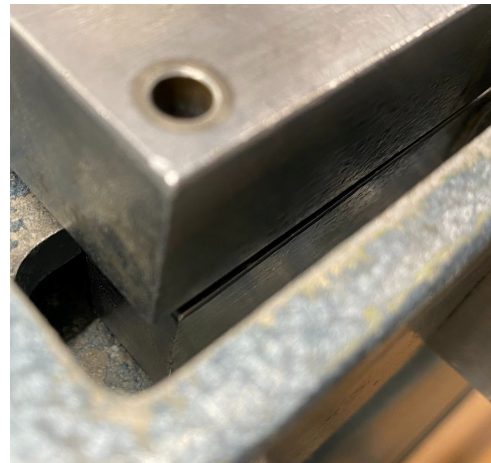
(b) Sample 1S during test. The inclination of the sample is demonstrated by the uneven space along the top and bottom of the sample holder.
