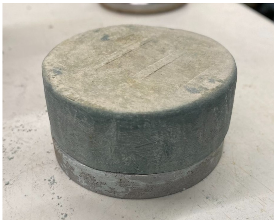
(a) Sample 1R-A after shear test.
