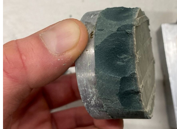
(b) Sample 2S. Still bonded to the steel disc after the end of the initial test.
