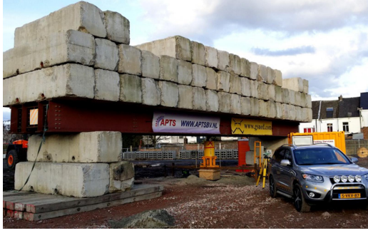
(a) Static load test setup (APTS 2021b, May 13).
