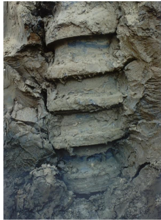
(b) Screw shaped (helical) shaft of pile Olivier Industrie (2021, April 5).
