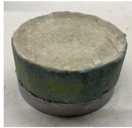
(b) Sample 4R after test. Only a very small amount of fracturing and chipping is visible.
