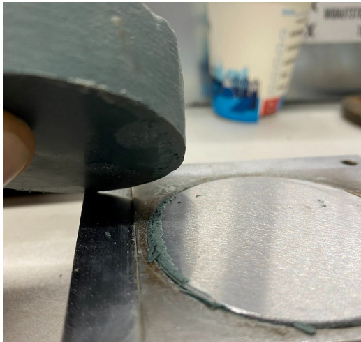
(a) Sample 1S after test. Note remaining grout of the edge of the steel plate, caused by the inclination.
