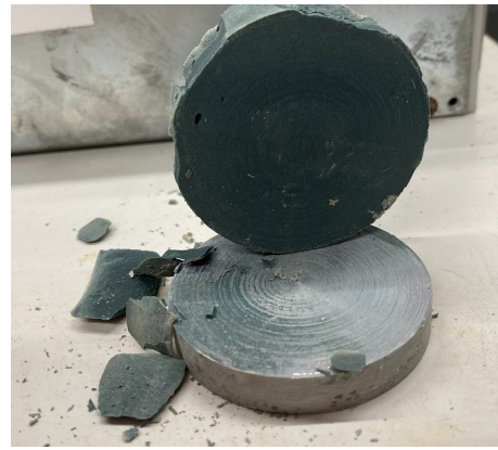
(b) Sample 2R after testing. Note the increased grout residue on one half of the steel disc, possible due to inclination of the sample.
