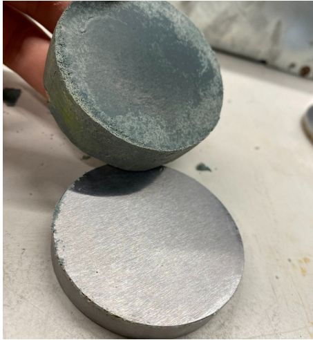
(a) Sample 4S after test. Note the shaving and grout residue on the left side of the sample.
