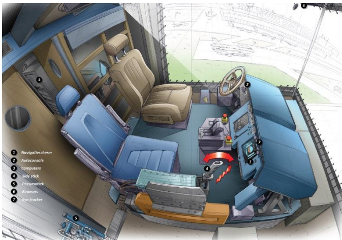
Figure 1: Illustration of HMI-Lab. The experiment will use the right side of the simulator, using the side stick and small display in front.
