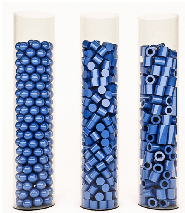
Fig. 2. Computer-generated structures using RBD algorithm for spheres, cylinders and Raschig rings with N = 4.1 , 4.58 and 4.05, respectively.
