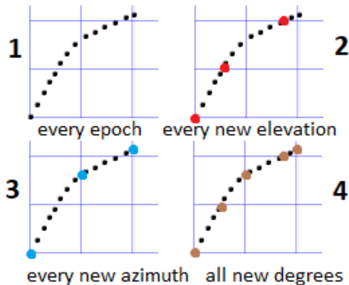
Figure 3.13: Examples of dealing with elevation and azimuth data. Vertical is the elevation angle and horizontal the azimuth angle
