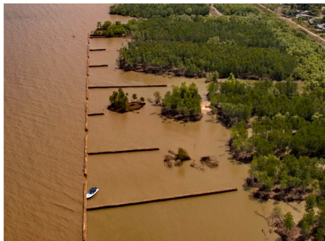
Fig. 16. Wave dampening effect of bamboo T-dams in Ca Mau Province, Viet Nam (courtesy R. Sorgenfrei, 2016).
