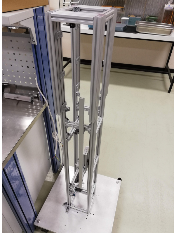
Figure 3.26: Frame made mostly out of extruded aluminum profiles.
