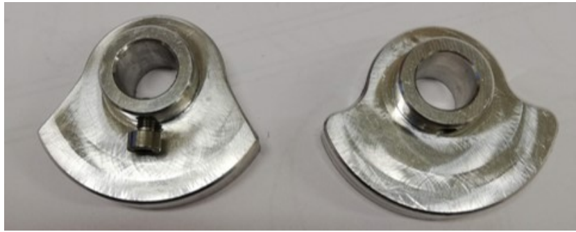
Figure 4.2: Original cam gear on the right with redesigned on the left.
