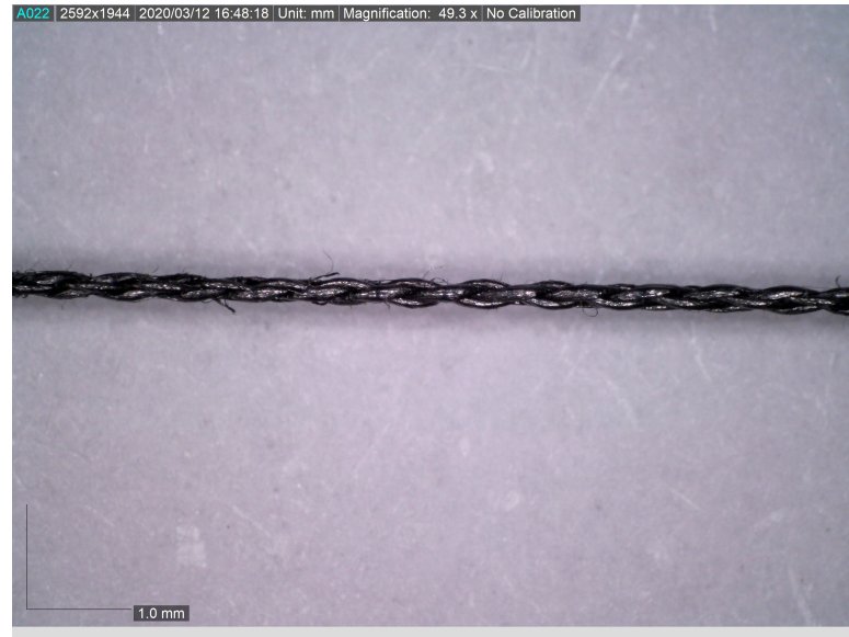
Figure 4.20: Carbon braided wires of 100 micro meters.
