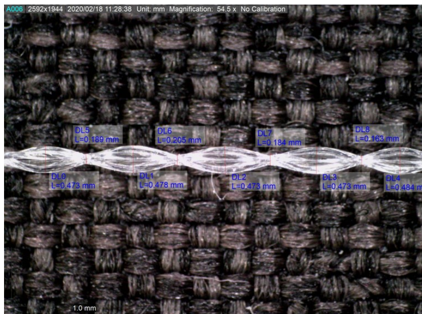
Figure 4.13: Nylon braided wires of 100 micro meters.
