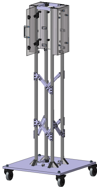
Figure 3.23: Frame design for the braiding machine.
