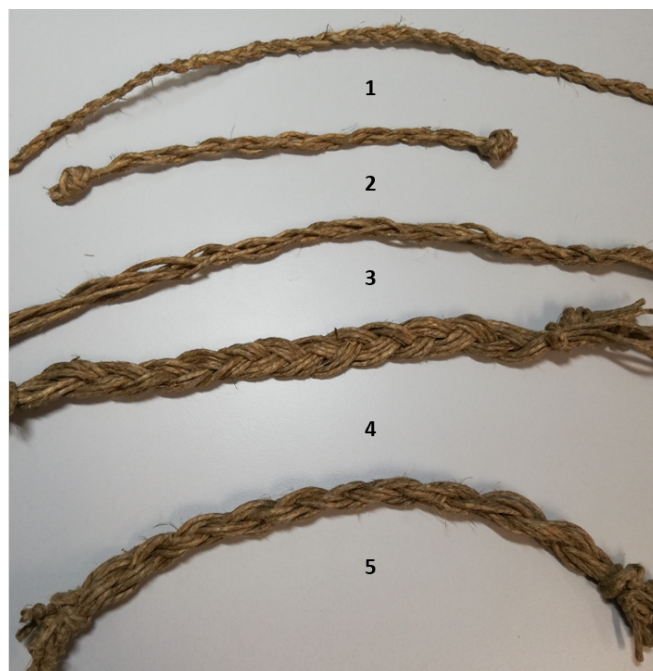
Figure 3.5: Prototype yarns created for better shape visualization. 1) 3x1, 2) 4x1, 3) 6x1, 4) 3x4 and 5) 4x3
