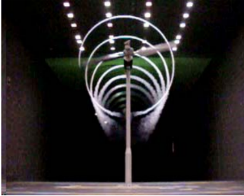
Figure 2.1: Spiral tip vortex line in the wake of a HAWT (Hand et al., 2001).
