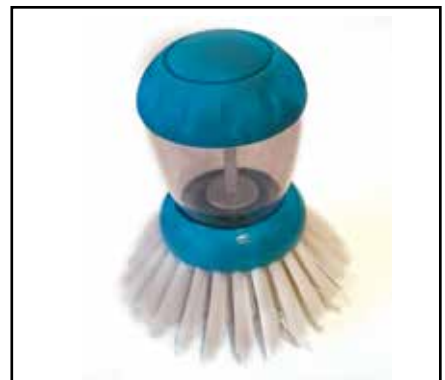
Figure 6.3 Brush ( \text{Ø } 85 \text{ mm} ) used to remove the biofilm from the concrete plates.
