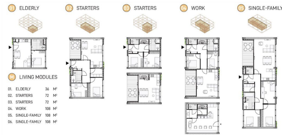
Figure 14: The system of the floorplans which offer different users a nice dwelling.
