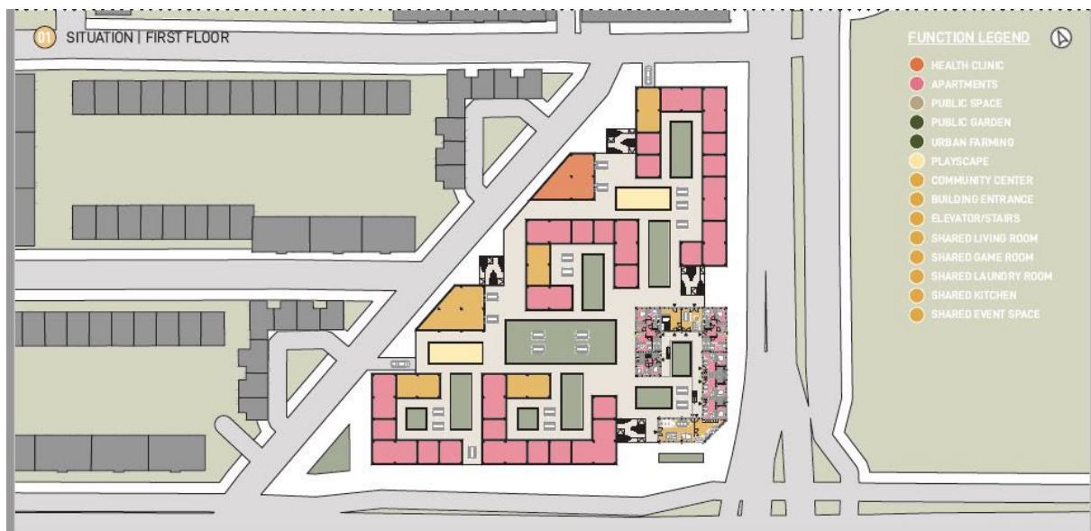
Figure 13: the ground floor. Each co-housing block has one community centre with a staircase, elevator and meeting rooms. The south/west corner offers a restaurant, at the north-east corner is a 'health clinic', which is meant as a neighbourhood health centre.
