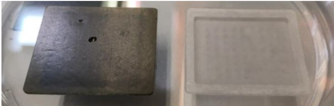
Figure A.3.2: Comparison of HTM140V2 (left) and 3DM Tough Clear (right) by printing flat plates (25 mm x 25 mm x 0.7 mm) that can be used as 2PP substrate for dose tests.
