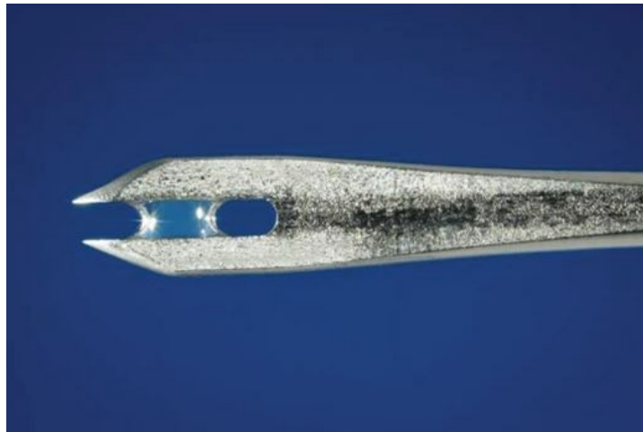
Figure B.9.60: Bifurcated needle which could be printed with at microscale for precise liquid handling. [22]
