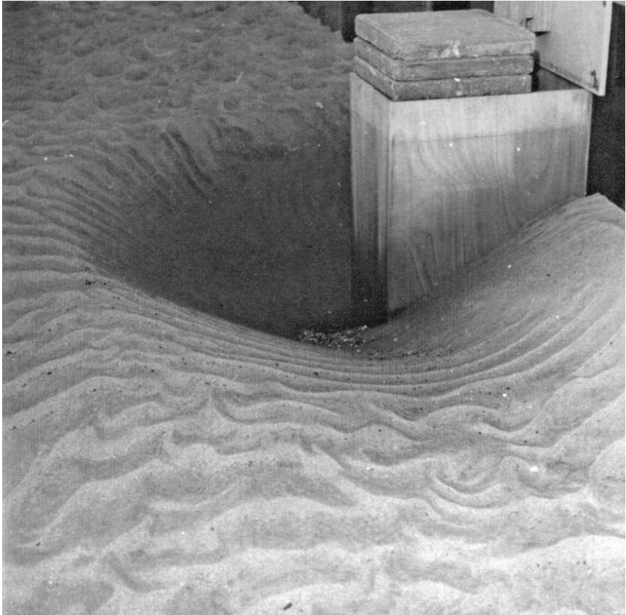
Scour in a horizontal constriction (photo Deltares)
