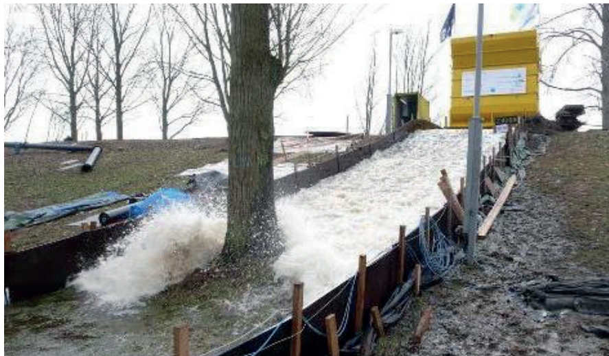
Figure 12-27 Overtopping Simulator (photo Infram)
