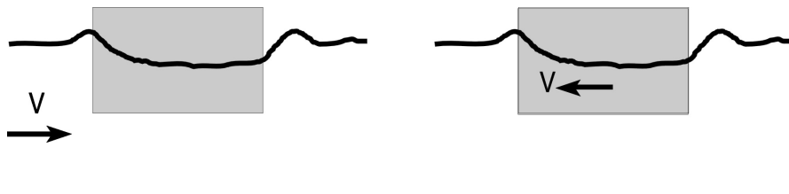
Figure 9-1 Flow around fixed object versus moving object in stagnant water
