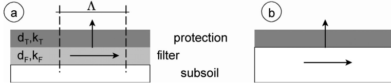
Figure 8-4 Definition leakage length
