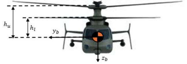
Figure 3: Front view of the compound coaxial helicopter.
