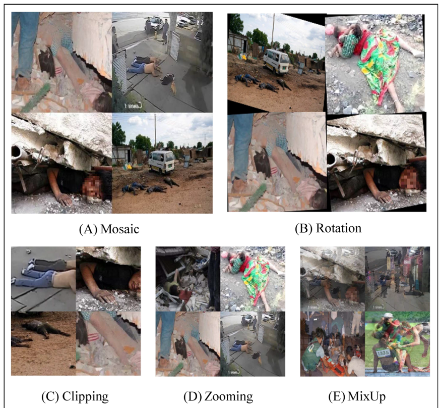
FIGURE 5 Partial images of train dataset after preprocessing: (A) Mosaic: Randomly select four images from the training set and put them into a synthetic image, (B) Rotation: Randomly rotate the images, (C) Clipping: Randomly clip the image size, (D) Zooming: Randomly zoom in/out images to various scales and (E) MixUp: Randomly mix different images and labels to generate new training data.
