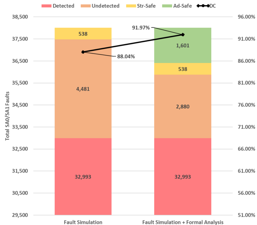
Figure 11. Combined results in CAN: uptrend in DC when fault simulation and formal analysis combined.
