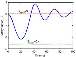
Fig. 7. Actual safety factor in speed regulation process.
