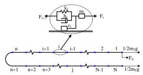
Fig. 4. Finite element model of belt conveyor.
