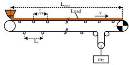
Fig. 5. Horizontal belt conveyor lay-out [19].
