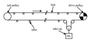
Fig. 3. Typical belt conveyor geometry [19].
