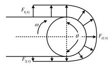
Fig. 1. Tensile forces exerted on the belt [19].
