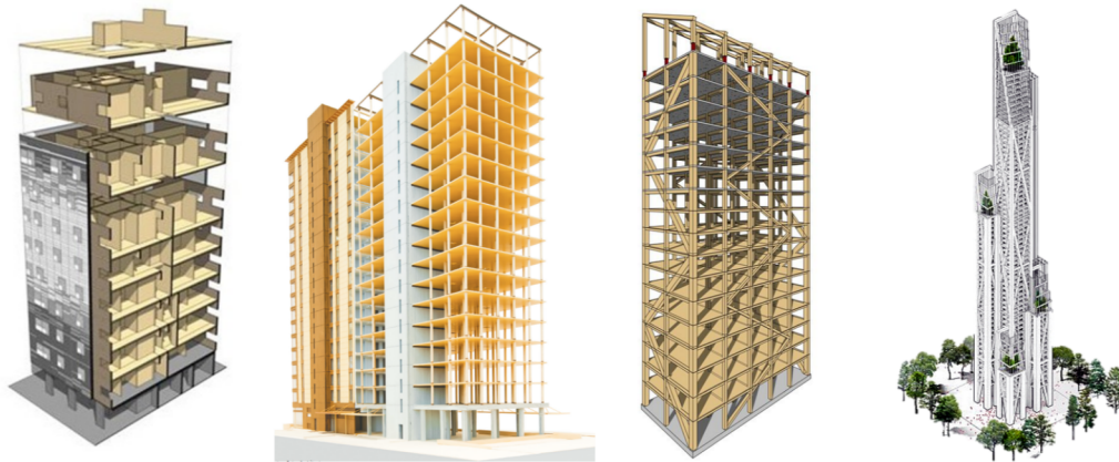
Figure 2.4: Examples of stability systems A) Shear wall [3] B) Core system [4] C) Tube system [5] D) Diagrid system [6]
