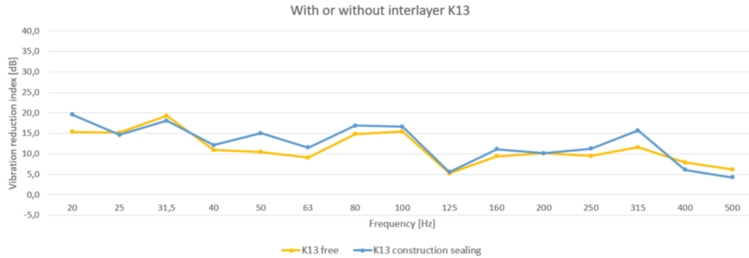
Figure 5.14: Results of the vibration reduction index K13 of a model without an interlayer and a model with an interlayer
