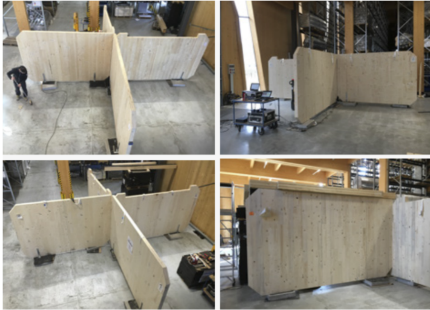
Figure 4.10: Vibration reduction index measurement set-up, the panels are resting on small concrete blocks to which they are connected with hold downs [24]
