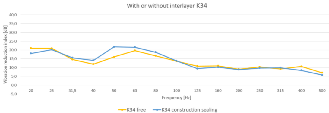
Figure 5.16: Results of the vibration reduction index K34 of a model without an interlayer and a model with an interlayer
