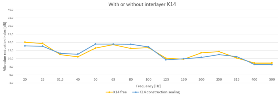
Figure 5.15: Results of the vibration reduction index K14 of a model without an interlayer and a model with an interlayer
