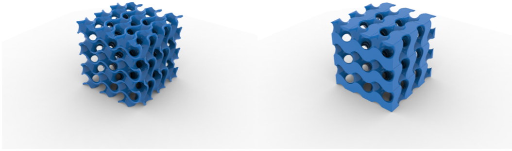
Figure 1.8: On the left sheet solid architecture of 2x2x2 Gyroid unit cells. On the right network solid with the same structure.
