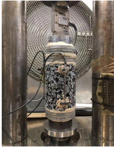
Figure 2.2 Setup for the temperature and frequency sweep test of PA mixes
