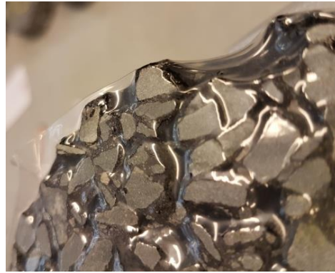
Figure 2.5 Plastic bags sucked into the air voids
