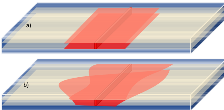
Figure 6.5. Schematic representation of the CCP specimen after fatigue-induced damages. a) Idealized, symmetric and straight crack evolution and b) realistic, unequal and non-straight cracks.
