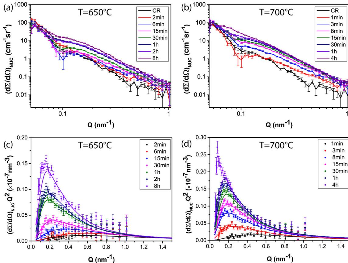
Fig. 7. Time evolution of  $(d\Sigma/d\Omega)_{\text{NUC}}$  as a function of  $Q$  measured at room temperature for samples annealed at (a) 650 °C, (b) 700 °C. Time evolution of  $Q^2(d\Sigma/d\Omega)_{\text{NUC}}$  as a function of  $Q$  after background subtraction of the CR sample for samples annealed at (c) 650 °C, (d) 700 °C, solid lines are the best fits using the model given by Eqs. (2) and (3).
