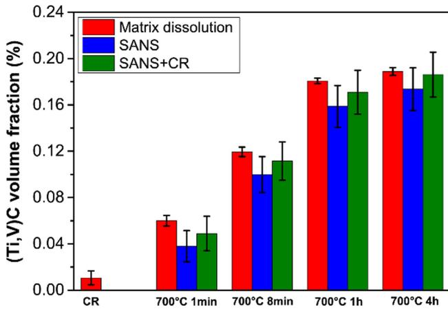
**Fig. 10.** Volume fraction comparison of (Ti,V)C precipitates obtained from matrix dissolution, SANS and SANS+CR. The “SANS+CR” means that the volume fraction in the CR sample obtained by matrix dissolution is added to the values obtained by the SANS measurements.
