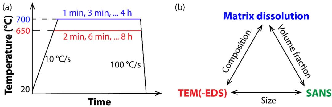
**Fig. 1.** (a) Schematic annealing procedure for the Ti-V HSLA steel samples, (b) precipitate size (distribution), composition and volume fraction are obtained by pairs of techniques including TEM imaging, TEM-EDS, matrix dissolution combined with ICP-OES and SANS.
