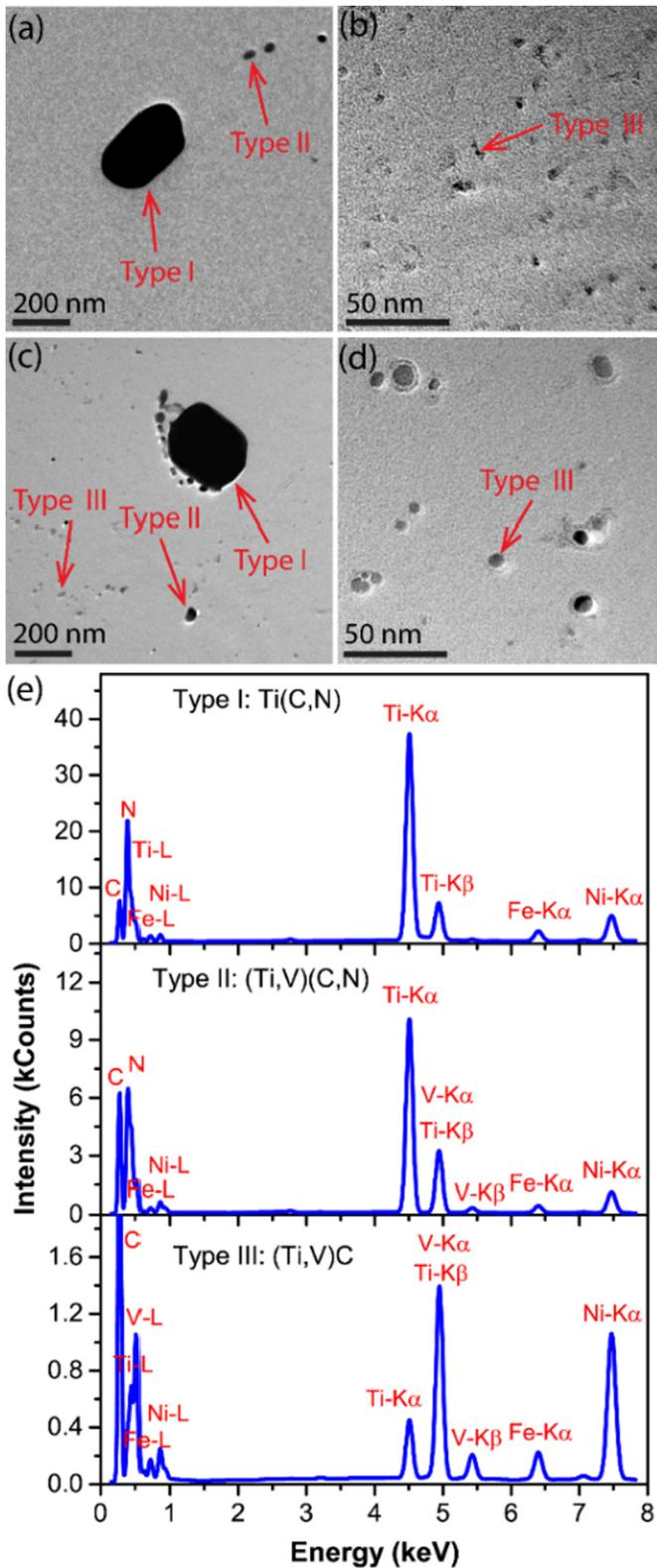
**Fig. 3.** Representative examples of bright-field TEM images of carbon replicas showing sizes and morphologies of the three different types of precipitates in the sample (a), (b) CR, (c), (d) 700 °C 4 h, and (e) EDS spectra of the three types of precipitates.
