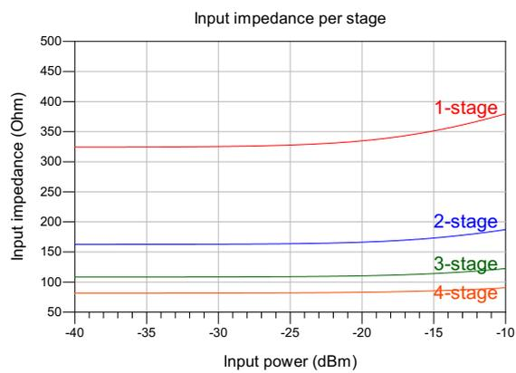
Figure 3.10: Input impedance for different stages
