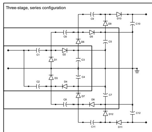
Figure A.4: Three-stage rectifier with series configuration
