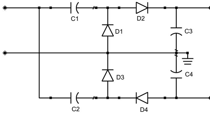
Figure 3.5: Schematic of a Greinacher rectifier.
