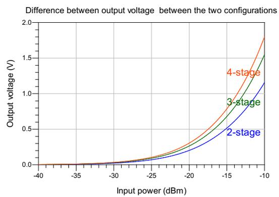
Figure A.12: Output voltage per stage with both configurations (parallel config.: solid line; series config.: dotted line)
