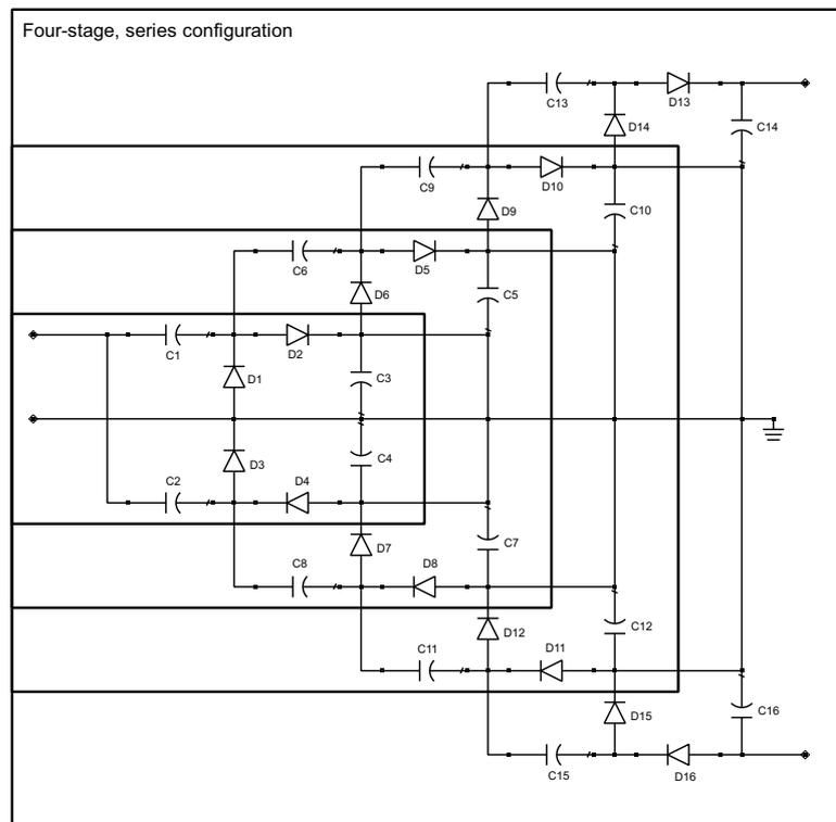
Figure A.6: Four-stage rectifier with series configuration
