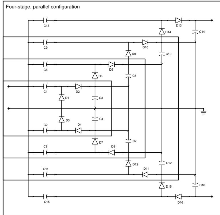
Figure A.5: Four-stage rectifier with parallel configuration
