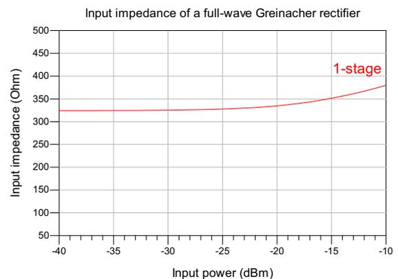
Figure 3.8: Input impedance  $|Z_{in}|$  for a single stage rectifier as function of input power
