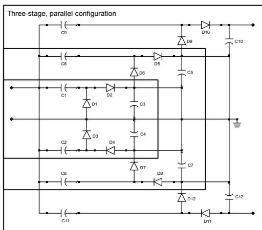
Figure A.3: Three-stage rectifier with parallel configuration
