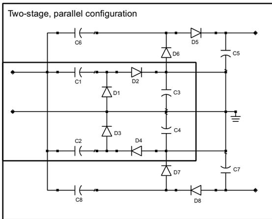
Figure A.1: Two-stage rectifier with parallel configuration
