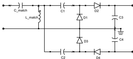
Figure 3.12: Greinacher rectifier with matching circuit
