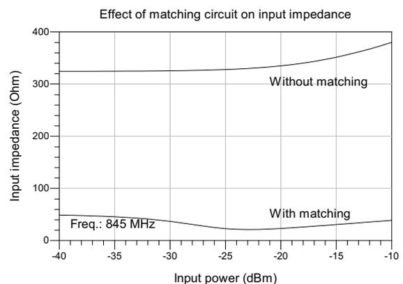
Figure 3.13: Effect of matching circuit on input impedance
