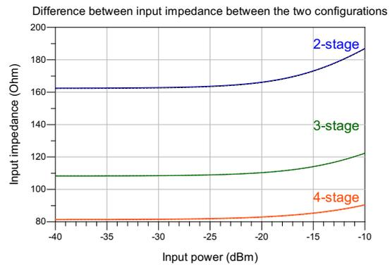
Figure A.8: Input impedance per stage with both configurations (parallel config.: solid line; series config.: dotted line)
