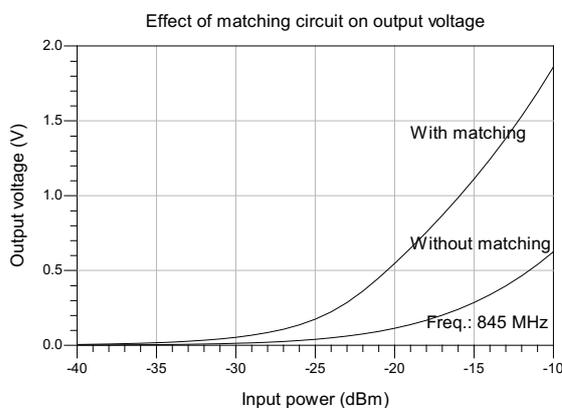
Figure 3.14: Effect of matching circuit on output voltage as a function of input power
