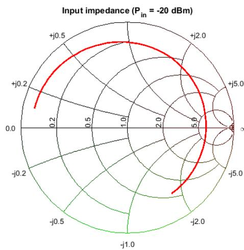
Figure F2: Measured input impedance from 800 MHz to 900 MHz at -20 dBm measured by a vector analyzer.
