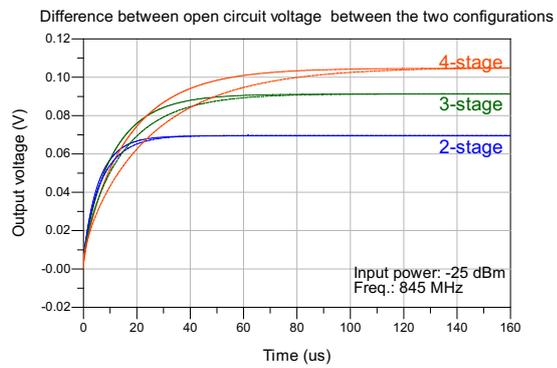
Figure A.10: Open circuit voltage with both configurations (parallel config.: solid line; series config.: dotted line)
