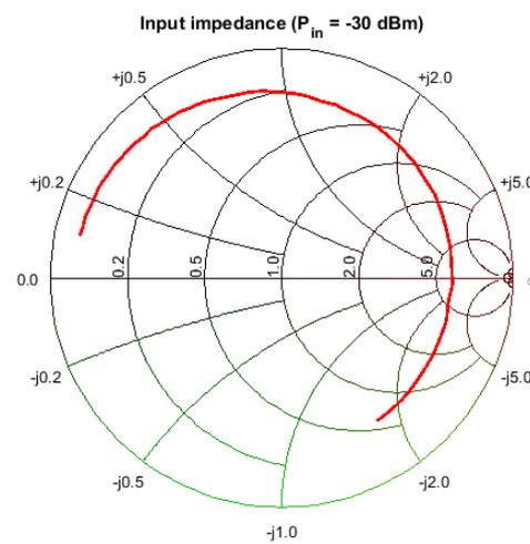
Figure F4: Measured input impedance from 800 MHz to 900 MHz at -30 dBm measured by a vector analyzer.
