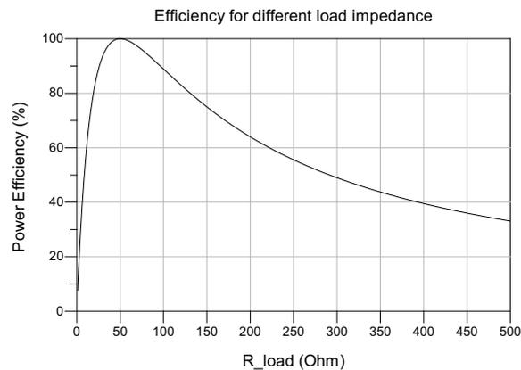
Figure 3.6: Efficiency of power transfer to the load for a  $50 \Omega$  source impedance.
