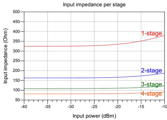
Figure A.7: Input impedance per stage with parallel configuration. It shows the 1-stage rectifier has the highest impedance
