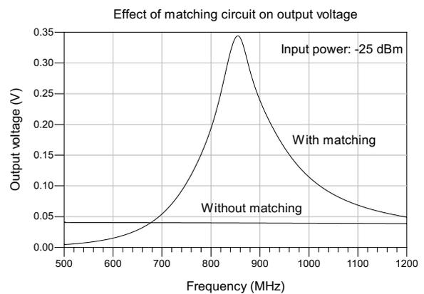
Figure 3.15: Effect of matching circuit on output voltage as a function of frequency
