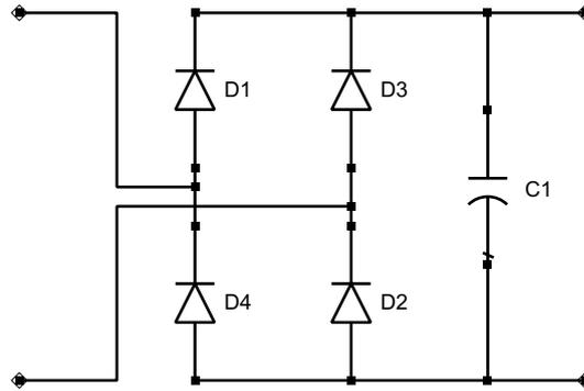
Figure 3.1: Schematic of a full-bridge rectifier.
