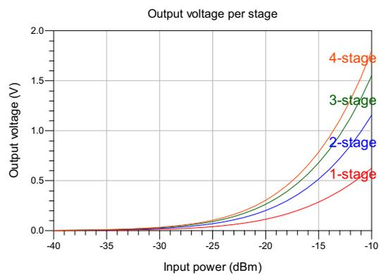
Figure A.11: Output voltage per stage with parallel configuration. All rectifiers are unmatched.
