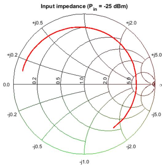
Figure 4.3: Input impedance from 800 to 900 MHz at -25 dBm as measured by a vector analyzer.
