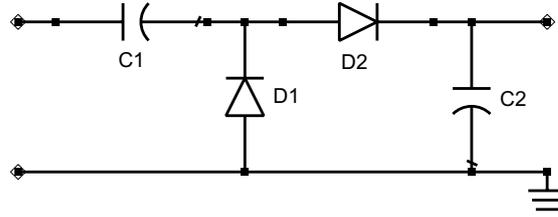
Figure 3.4: Schematic of a Dickson rectifier.
