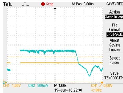
Figure 4.2: The output voltage as a phone in close proximity of the antenna was being called. The blue line represents the output of the rectifier, and the yellow line is the output of the DC/DC converter. Here the x-axis represents the time (1 sec per square) and the y-axis represents the voltage (1.0 V per square for CH1, 500 mV per square for CH2)
