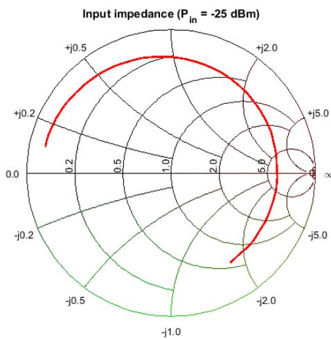
Figure F3: Measured input impedance from 800 MHz to 900 MHz at -25 dBm measured by a vector analyzer.
