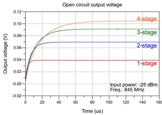
Figure A.9: Open circuit output voltage per stage with parallel configuration. All rectifiers are unmatched.
