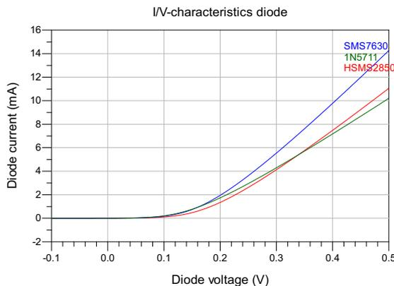
Figure 3.2: DC-characteristics of Schottky diodes
