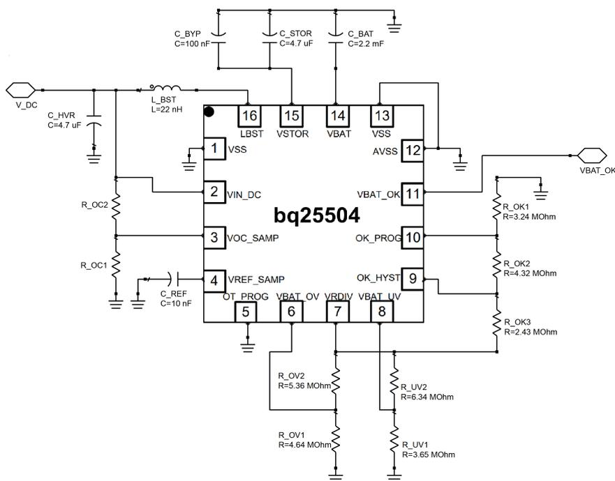
Figure 3.16: Schematic of a the BQ25504 with configuration components
