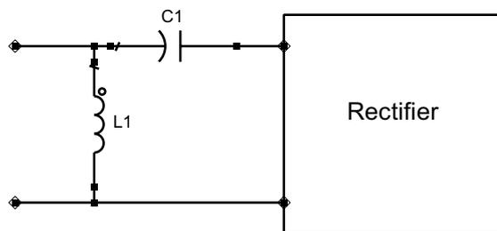
Figure 3.11: Schematic of a resonator.
