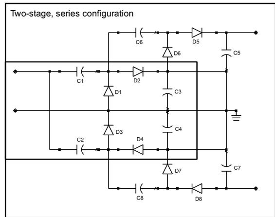
Figure A.2: Two-stage rectifier with series configuration
