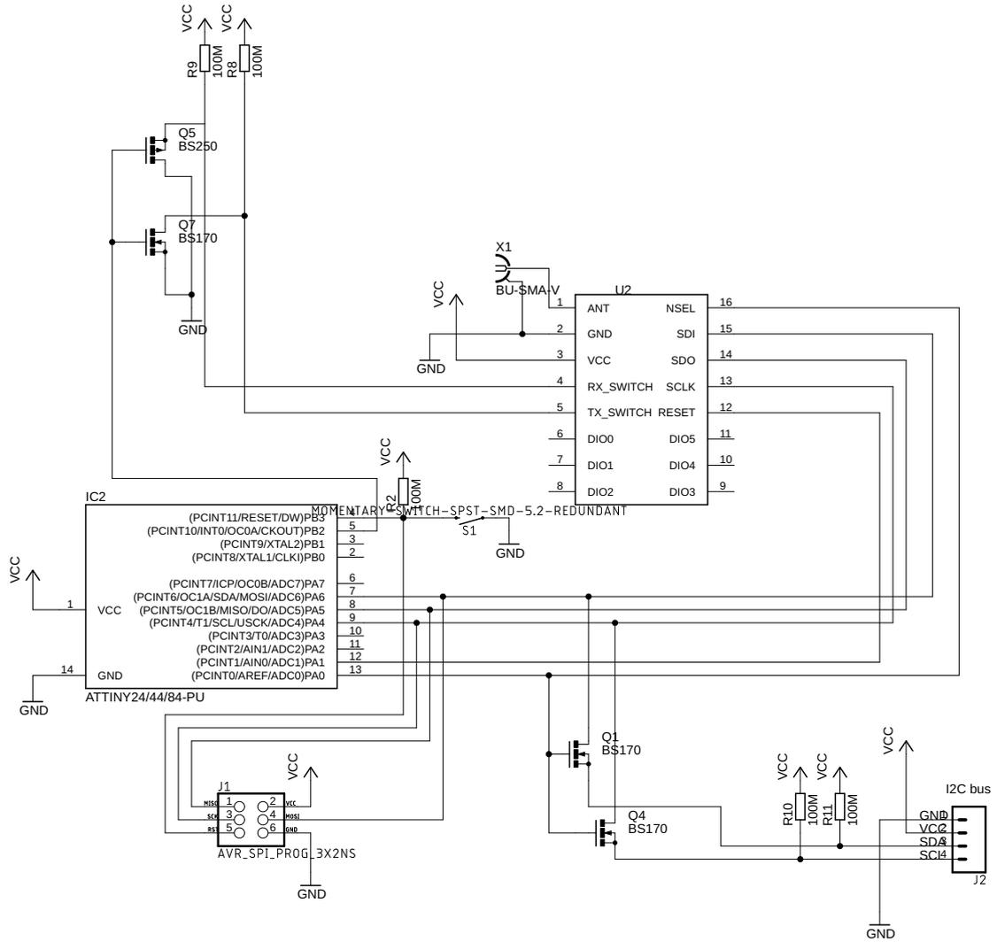
Figure E.2: The PCB design of the sensing and communication subsystem
