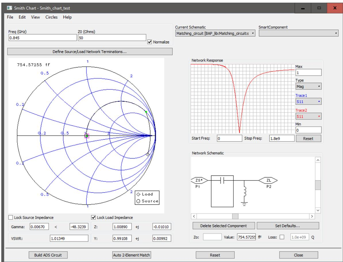
Figure B.1: Smith Chart of the matching circuit. The inductor and capacitor shift the input impedance to the midpoint of the graph, which is equal to 50 Ohm.
