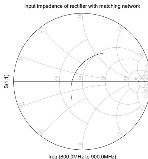
Figure 4.4: Input impedance from 800 to 900 MHz at -25 dBm as simulated with ADS
