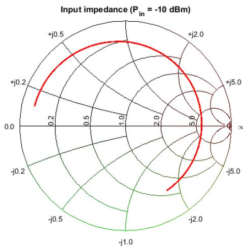
Figure F1: Measured input impedance from 800 MHz to 900 MHz at -10 dBm measured by a vector analyzer.
