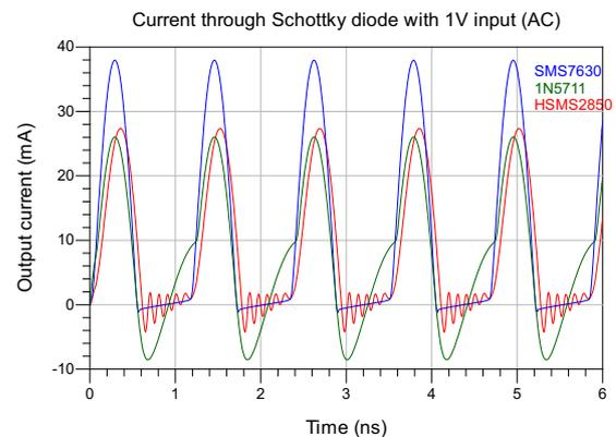
Figure 3.3: AC-characteristics of Schottky diodes
