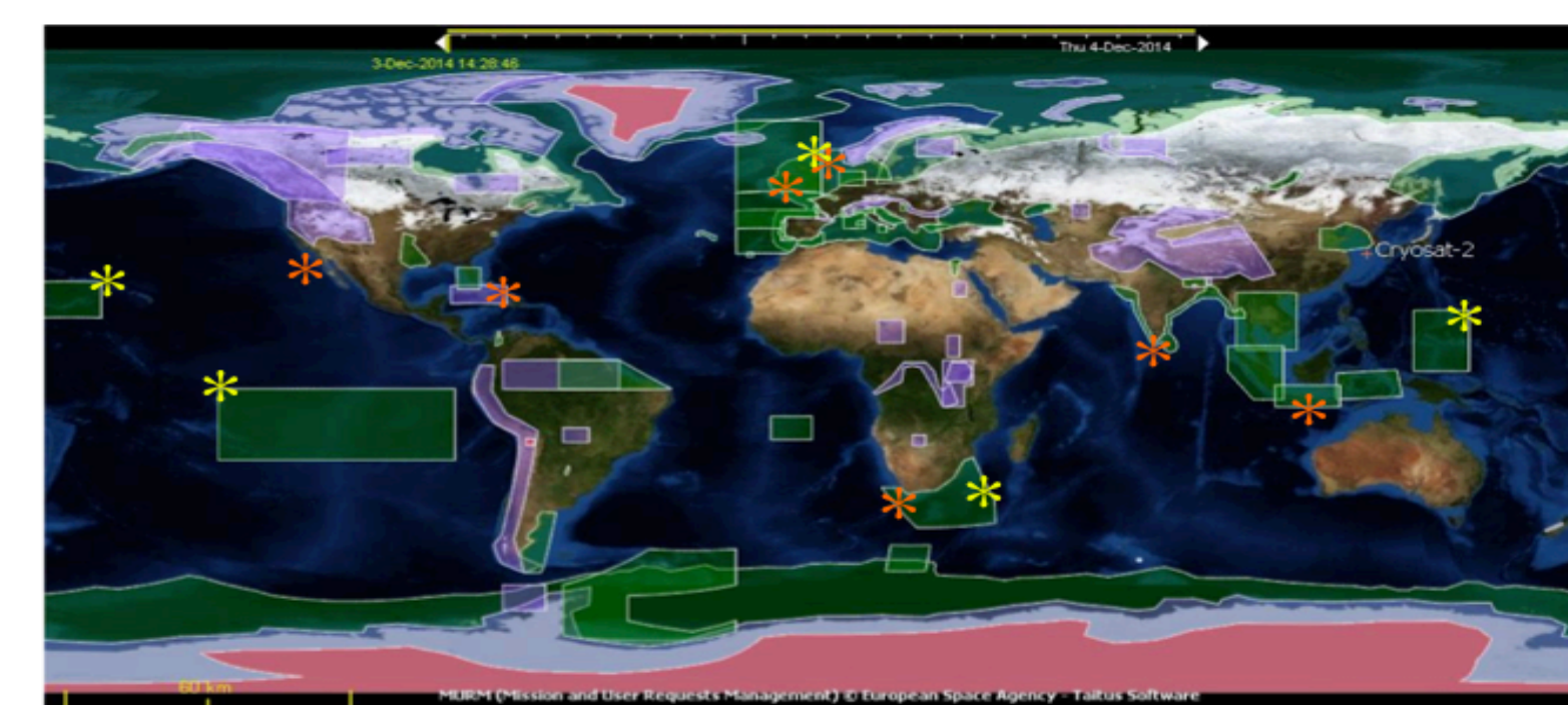
Figure 1 Regions included in the SCOOP study, based on a CryoSat SAR mode mask figure from ESA, with yellow indicating open ocean areas and orange coastal areas (note the Northeast Atlantic and Agulhas regions are assigned to both)
