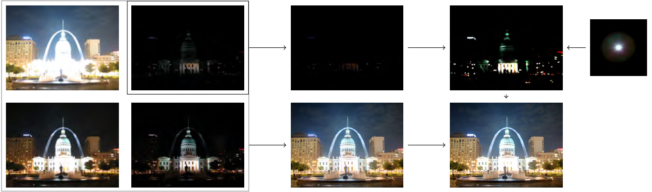
Figure 4: A complete overview of the tone map and bloom method. Given as input are pictures with multiple exposures, which are combined into a tone mapped image using Merten’s Exposure fusion [10]. The picture with the lowest exposure rate is taken to create the bloom effect. It is smoothed first, then convolved with a kernel. The tone mapped image and the bloom overlay are combined into a final image. Original images by Kevin McCoy [4].
