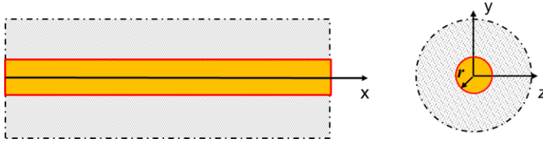
Figure A2. Schematic for the structure of metal line laterally confined in elastic matrix.
