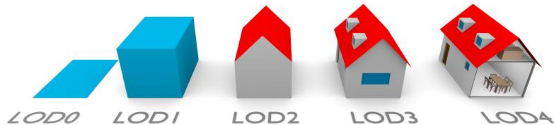
Figure 9: LOD in CityGML [Biljecki et al., 2017].
