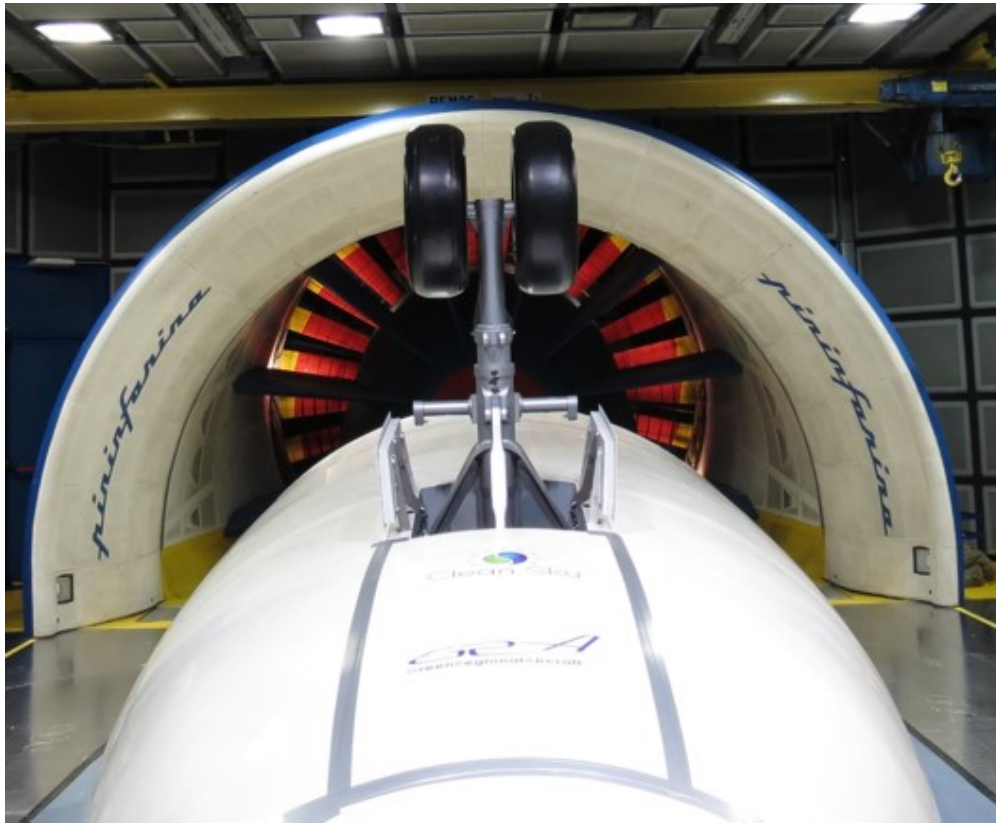
Figure 3: ALLEGRA NLG model inside the wind tunnel.
