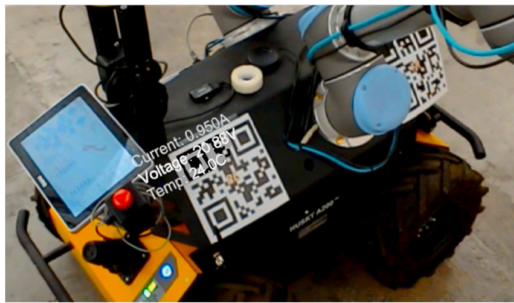
FIGURE 16. Mixed reality interface showing natural language of the health status of the robotic platform via the corresponding QR code.
