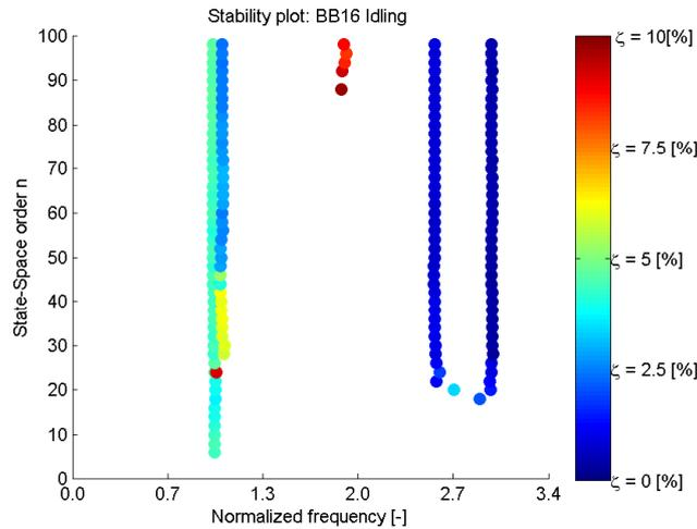
Figure 4: Example of a stability diagram obtained from measurement data acquired at an average wind speed of 1.7 m/s. Note that the damping values are shown in percentage of critical. (source: [8])
