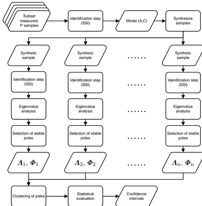
Figure 2: Flowchart of the applied Bootstrapping approach.
