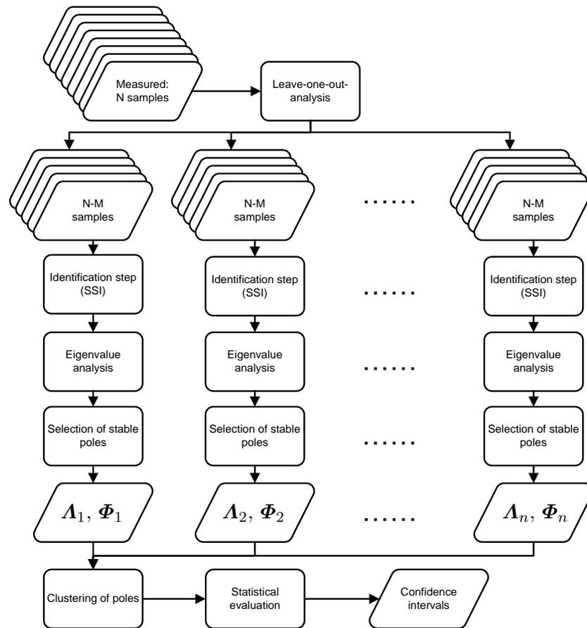
Figure 3: Flowchart of the approach based on the *leave-one-out* analysis.
