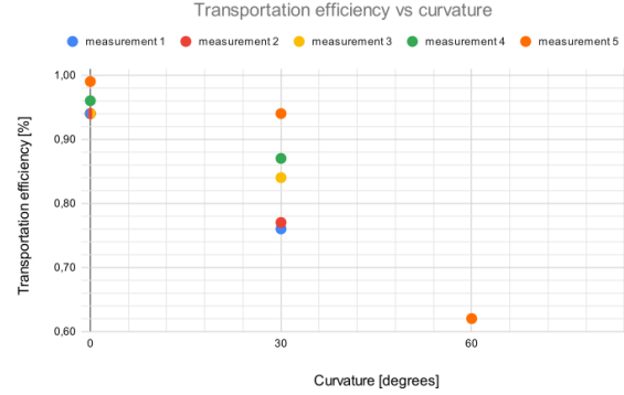
Fig. 28: Scatter plot displaying the influence of shaft curvature on transportation efficiency. Overlapping measurements are shown as multicoloured circles.
