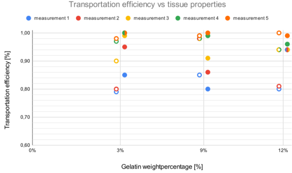
Fig. 27: Scatter plot displaying the influence of tissue properties on transportation efficiency. Measurements for the half-cylindrical phantoms are denoted by hollow circles, the cylindrical phantoms are denoted by full circles. Overlapping measurements are shown as multicoloured circles.
