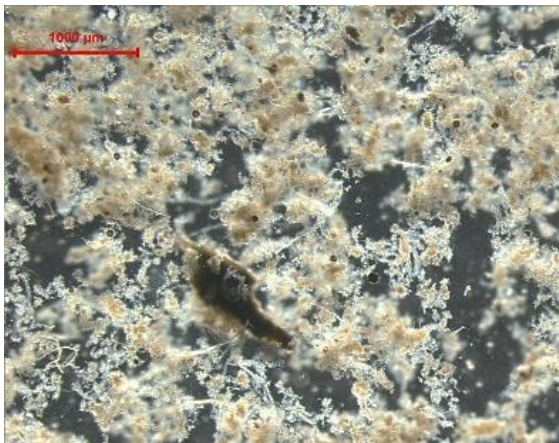
Figure 3. Microscopic picture of untreated Nereda® Excess Sludge collected at Garmerwolde STP, showing mainly sludge, fibres and other debris (scale bar 1000 µm).
