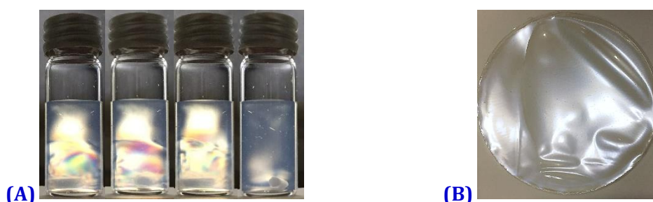
Figure 14. (A) Time lapse showing the dynamic birefringence in a suspension of isolated CNCs (MCC), between cross polarizers. (B) Thin film casted by air-drying CNCs from MCC after ultrasonication. The film shows light blue structural colour due to the ordering of CNCs (pitch was developed).
