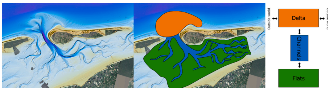
Fig. 2. Schematization of a tidal inlet system into a 3-elements ASMITA model, with the ebb-tidal delta, channel and flats (Lodder et al., submitted).
