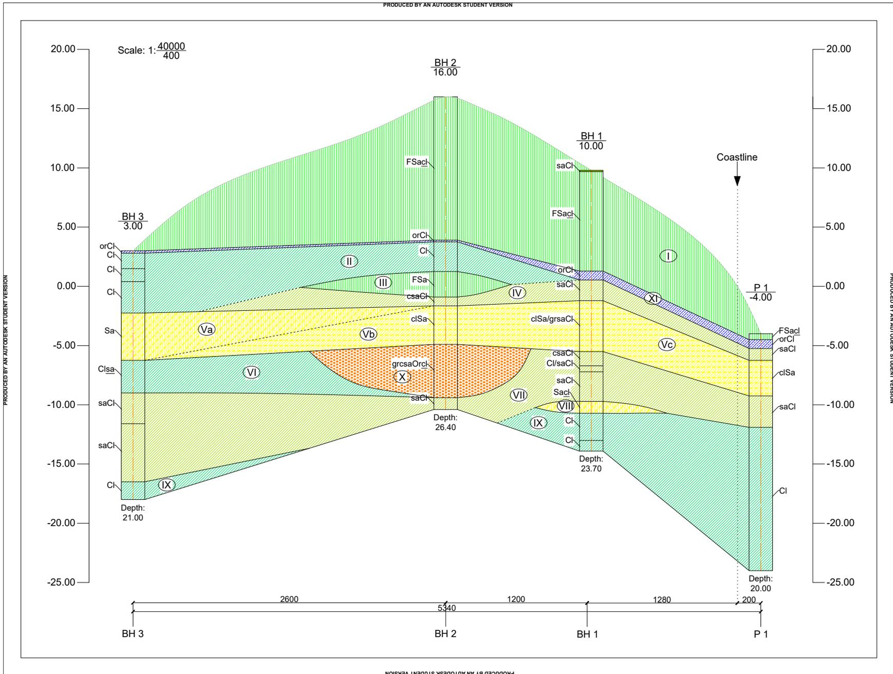
Figure C.1: Stratigraphy of Pinamar (noted scale is based on a full size A4 format)
