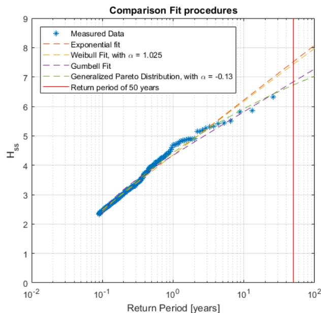
Figure 3.15: Example of extreme wave analysis of wave rose 3 for zone B
