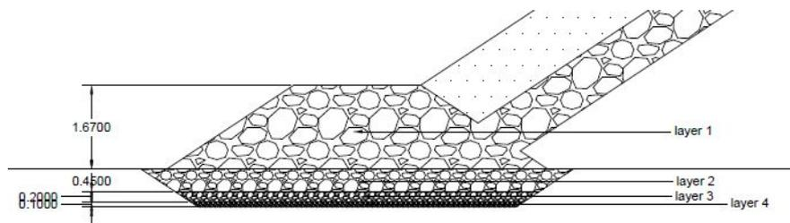
Figure 7.7: Cross section toe structure of the breakwater
