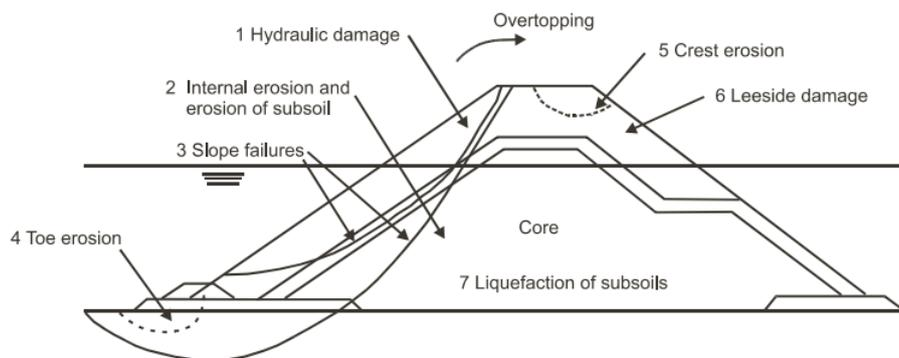
Figure 7.2: Rubble-mound breakwater failure modes [71]
