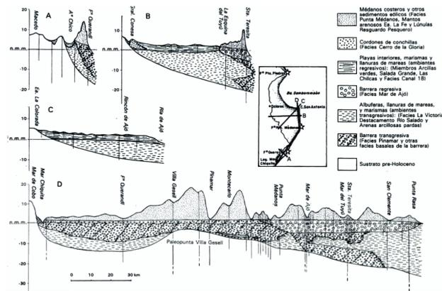
Figure 3.26: Stratigraphic cuts typical of different sectors of the Buenosairean coast [73]
