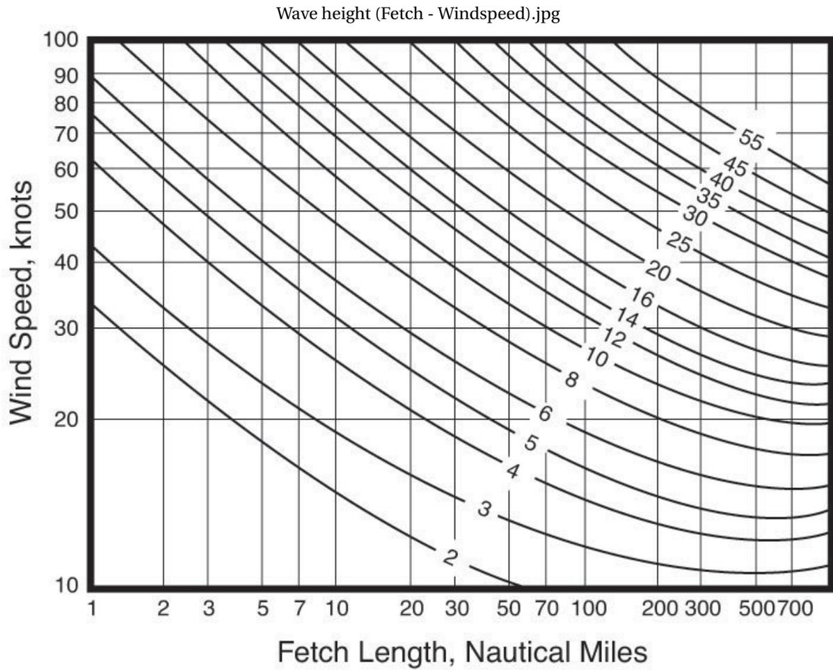
Figure F1: Windspeed vs Fetch
