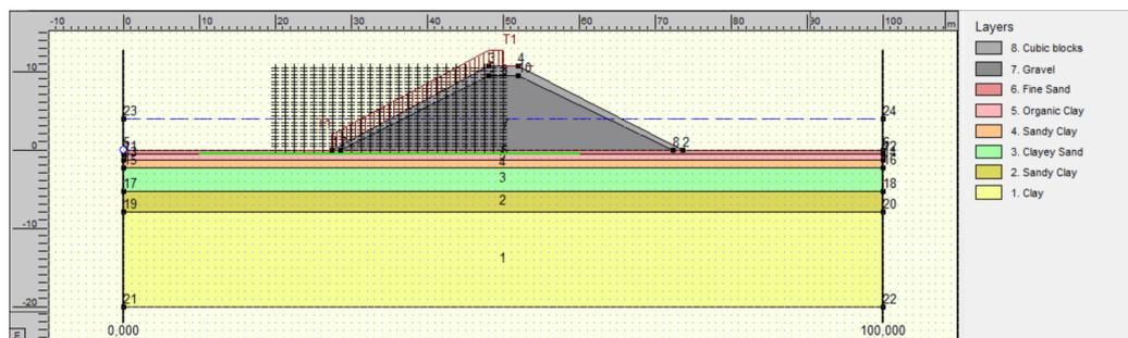
Figure 7.4: Numerical model for the slope stability of the breakwater
