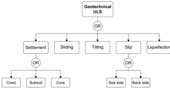
Figure 7.3: Geotechnical part of the fault tree for limit states of rubble-mound breakwater [22]
