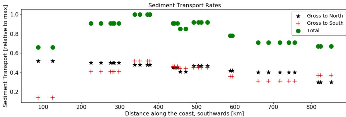
Figure 3.27: Gross and total sediment transport rates
