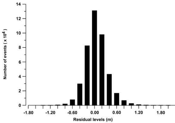
Figure 6.1: Measured residuals for the period 1956 - 2005, hourly measurements [24]
