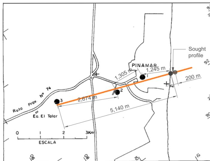
Figure 6.3: Modified map of the geological drillings in the Pinamar area [55]
