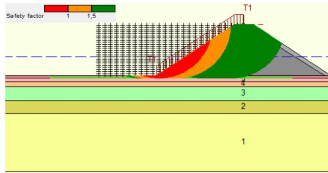
Figure 7.5: Strength reduction factor distribution for the breakwater with slopes of ratio 1:1.5
