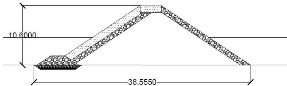
Figure 7.6: Cross section breakwater design
