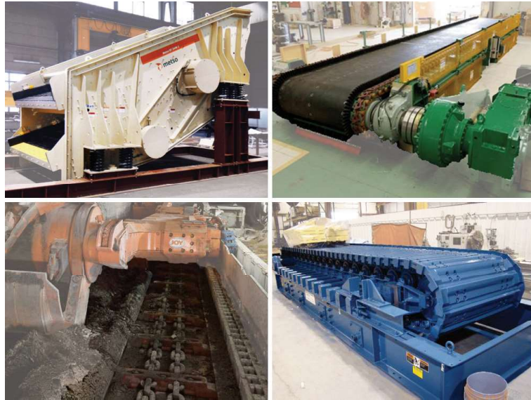
Figure 3.3: Top: Vibratory feeder [23](left), Low profile feeder [34](right), Bottom: Chain conveyor [17](left), Apron feeder [23](right)
