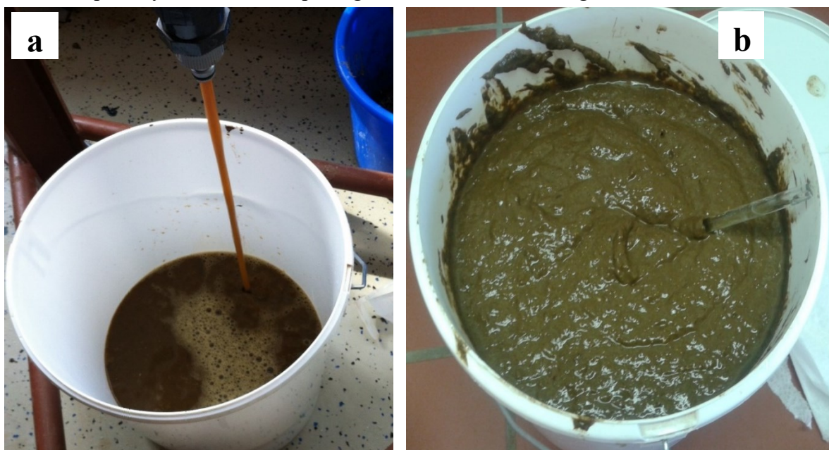
Figure 5-2. (a) Blackwater and (b) blackwater FS (sludge cake) obtained after centrifugation (Photo: P. Mawioo)
