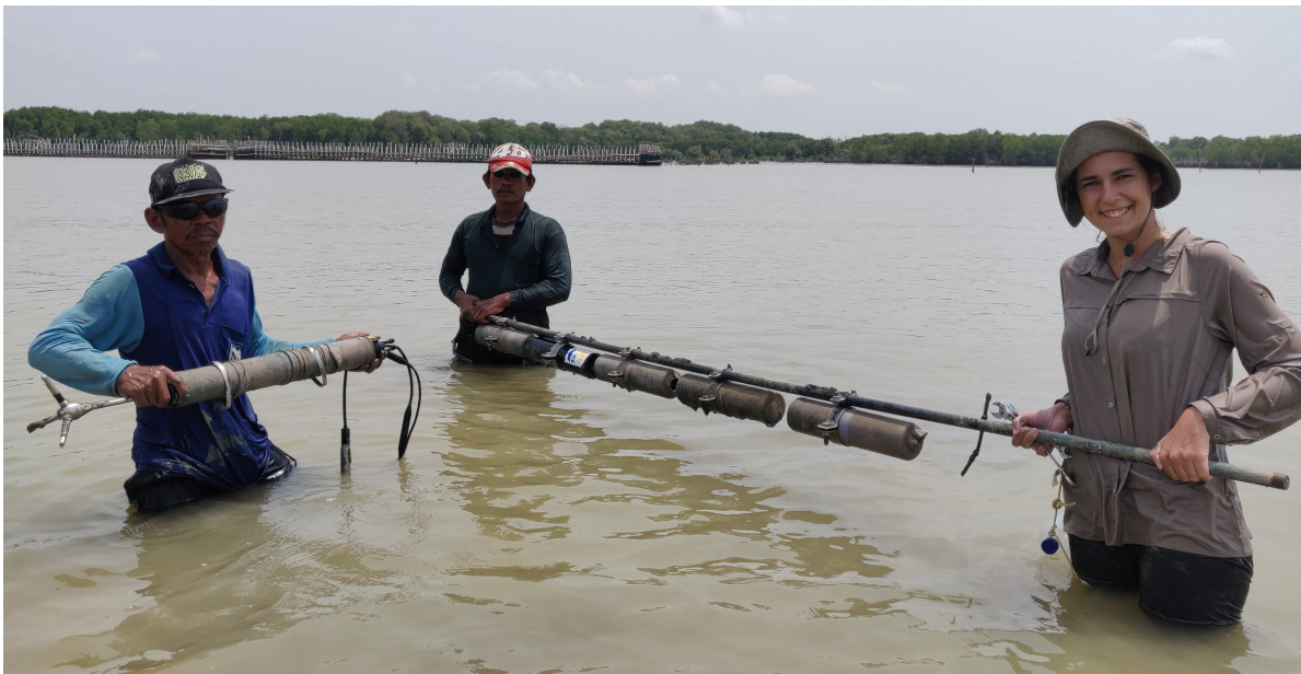
Figure C.1: Waveloggers mounted for calibration. The pole to which the instruments were attached was placed on the bottom for 5 min. The water depth during this period is known. To synchronise the internal clocks of the instruments, the pole was submerged 3 times in a fast sequence.
