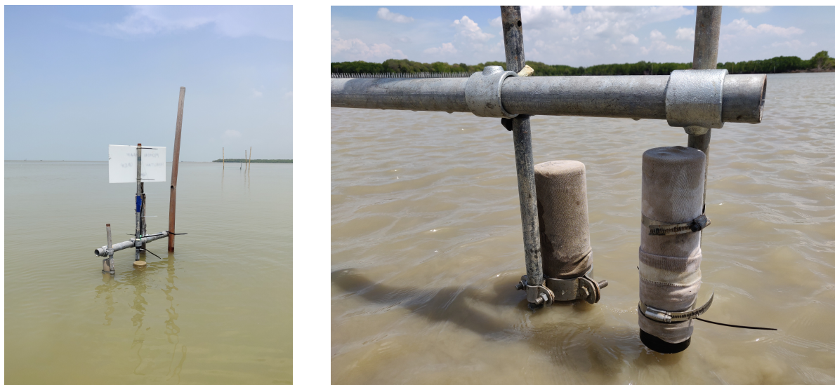
(a) From left to right; echologger, wave gauge, ADV
