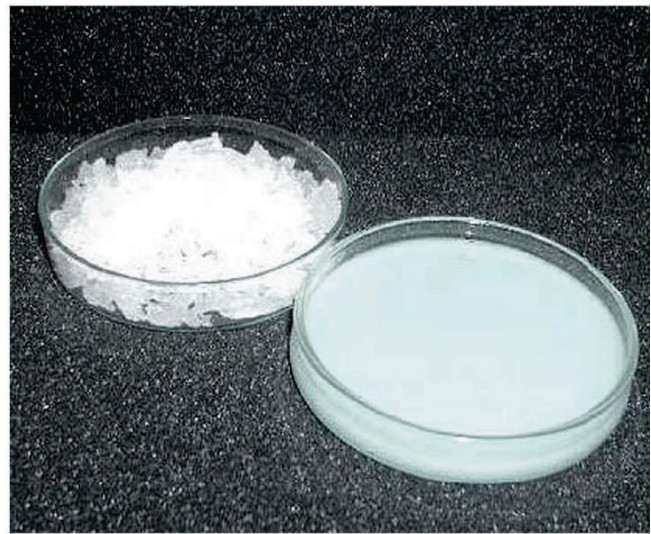
Fig. 2.20, The image indicates Parafin wax and salt hydrates PCM Source: Building Physics lecture notes 3, TU Delft, Aart Schuur and Wim van der Spoel
