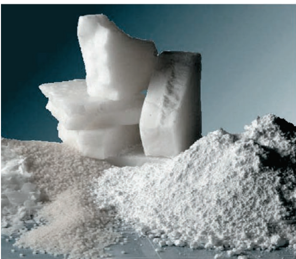
Fig. 2.20, The image indicates Parafin wax and salt hydrates PCM Source: Building Physics lecture notes 3, TU Delft, Aart Schuur and Wim van der Spoel
