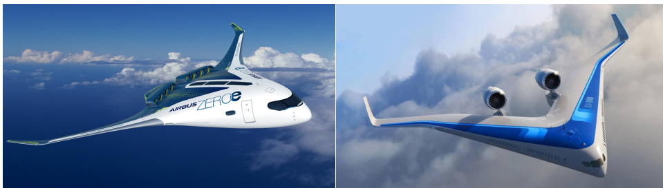
a) Airbus ZEROe BWB concept (© Airbus)
