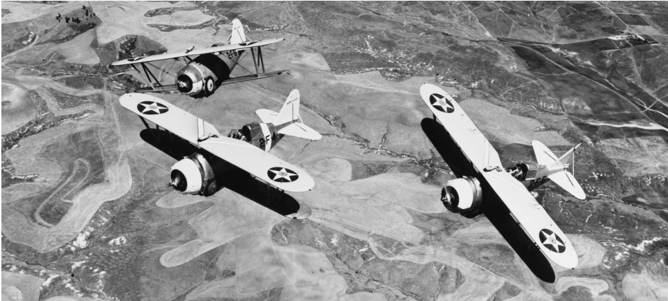
Figure 6.1 Three Northrop Grumman F2F-1 fighters in steady, aerobatic, formation flight, 1939 1 . The leader is trimmed in straight and level flight, while the followers are trimmed in steady, asymmetric flight with forward slip.
